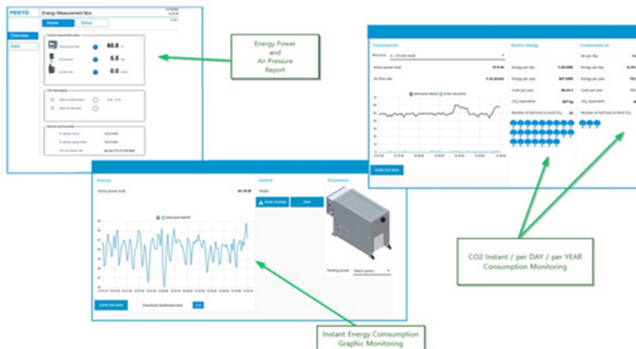
Figure 3.6 - Setup 6 - Energy parameters
